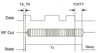
The transition from transmission to sleep state is handled automatically: the module waits for TOFFT idle time (4) on the pin TX DATA before returning to the sleep state.
