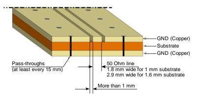
Note: dimensions in the picture above is referred to a FR4 substrate PCB
