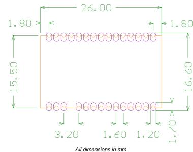
Neither via-holes nor wires are allowed on the PCB upper layer in area occupied by the module.
