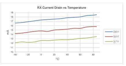
(\*): Consider all graphs as indicative typical results in accordance with temperature variation. Values measured with continuous wave transmission, max power, load 50  $\Omega.$
