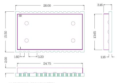
ALL DIMENSIONS ARE IN MILLIMETERS GENERAL TOLERANCE +/-0.1MM
